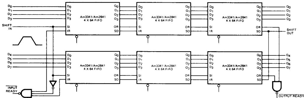
The composite input ready indicates both devices are ready to receive data. The shift in pulse must be wide enough for all devices to load data under worst case conditions.
