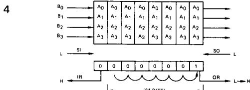
Data spontaneously ripple through registers to end of FIFO, causing OR to go HIGH. The time required for data to fall completely through the FIFO is the "Ripple-through Time".
