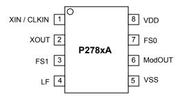
Standard pin Configuration offered in both 8 pin SOIC and TSSOP Packages
