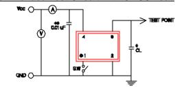
\* CL (Capacitive Load): Includes the input capacitance
