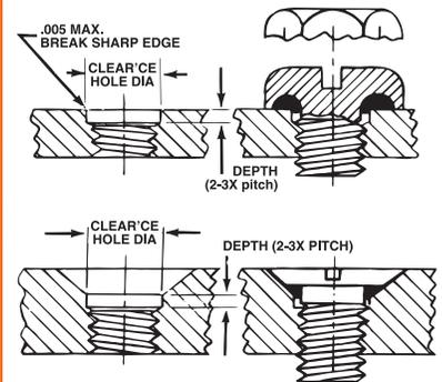
To assure maximum sealing performance of SEELSKREWS® and SEELBOLTS® a clearance hole must be used.
